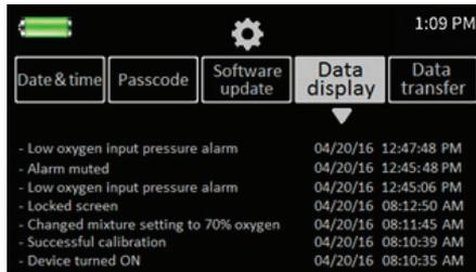
The mixer will store any event including all alarms and their related actions, turning the device ON or OFF, pressing the Oxygen Flush key, setting changes after confirmation, activating and canceling the alarm silence, calibration results, software updates as well as locking and unlocking the screen.
