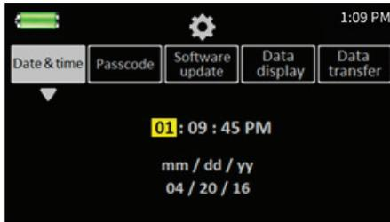
To increase the setting, rotate the knob clockwise. Rotate it counter-clockwise to decrease it (except for the AM/PM cell where the direction of rotation does not matter). Press the Control Knob (K) to confirm the change.
