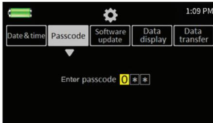
After entering the new passcode, a second line will appear beneath the first, prompting the user to confirm the new passcode.
