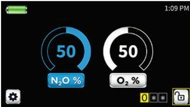
To activate the lock feature, rotate the Control Knob until the selection frame on the display screen surrounds the lock symbol, as shown in the picture.
