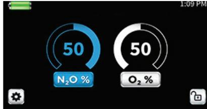
Once the operation screen is displayed with all the relevant parameters, the eAdvantage® mixer is ready for operation.
