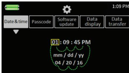
Use the Control Knob (K) to move this square frame to the particular cell (e.g., hour, minute, day, month, year) you want to change. The green dotted lines shown above indicate the sequence for selecting each cell based on the rotation of the Control Knob.
