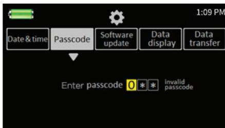
If the entered Passcode is accepted the screen will change to prompt the User to enter the new passcode otherwise it will show "invalid passcode" and the operator must repeat the above steps or select "Cancel" to exit without changes.
