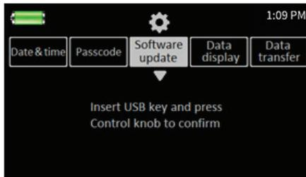
Upon inserting the boot loader USB key into the eAdvantage® system, the confirmation indicator light (J) will start flashing, indicating the need to confirm the selection manually before initiating the software update process.
