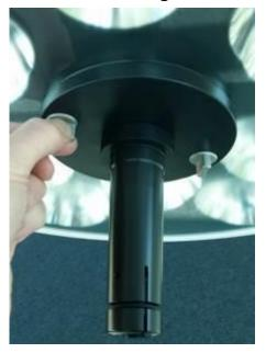
The camera can be attached to the lamp body in place of the handle unit.
