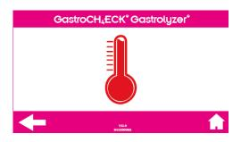
The temperature of the GastroCH₄ECK® Gastrolyzer® is above 25°C and is too hot to be calibrated. Please move the device to a cooler area and try again later.
