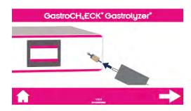
The device will then illustrate to attach the breath bag. Ensure to carefully remove the blue plug on one end only and attach the bag to the moisture filter, then open the clamp on that end only to preserve the sample.
