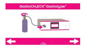
Attach the CaliAdaptor to device via the sample line and open the gas canister. Press the arrow to begin the calibration.
