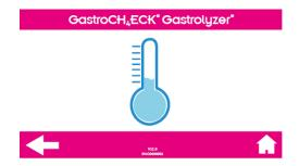
The temperature of the GastroCH<sub>4</sub>ECK® Gastrolyzer® is below 17°C and is too cold to be calibrated. Please move the device to a warmer area and try again later.
