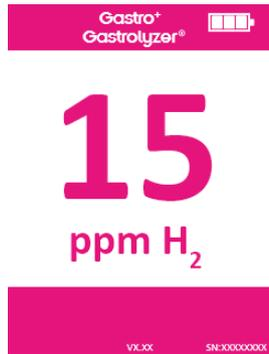
The ppm levels will rise and hold at the peak level, when this has stopped rising for a period of 5 consecutive seconds the test result can be recorded and the test stopped.
