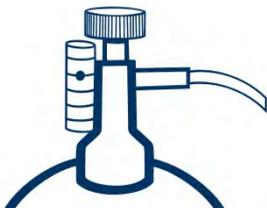
Allow the gas to flow at 0.5 litres per minute.
