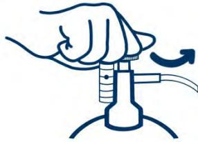
Allow the gas to flow through the instrument for the duration of the test, again monitoring the rate of flow.
