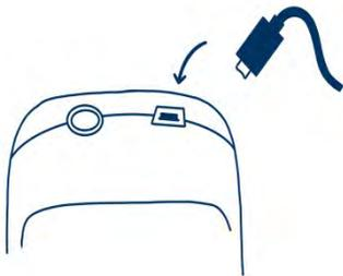
Place one end of the connection lead into the USB socket on the top of the Gastro<sup>+</sup>™ Gastrolyzer<sup>®</sup> product.
