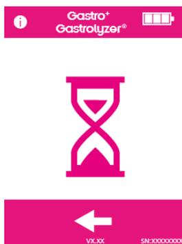
If the timer is shown, the sensor is stabilising.
