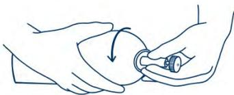
Screw the fine control valve and flow indicator assembly to the gas can. This is best done by screwing the gas can into the valve.
