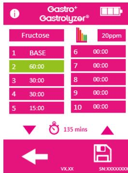
Select up to 10 time intervals by pressing the interval slot and increasing/decreasing the up or down arrows.
